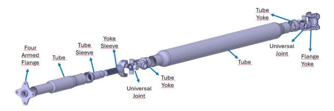
Figure 1 Propeller shaft
