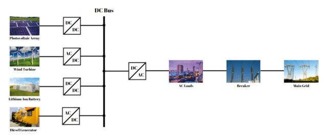
Fig. 1. Block diagram of the designed DC MG system
