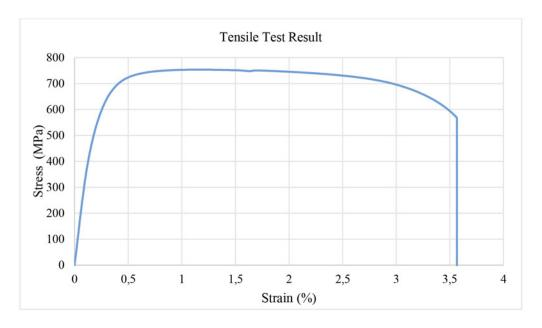
Figure 4 Strain-stress curves of the tube sample
