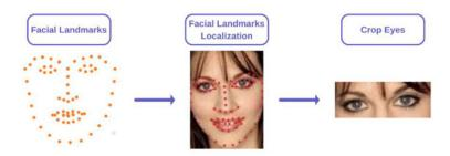
Figure 5. Cropping Eyes from Images with Face Landmark Detection
