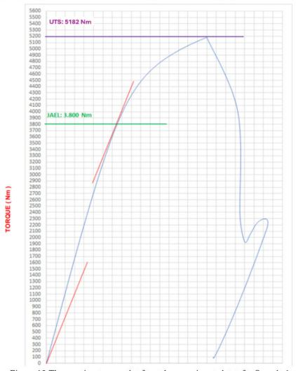
Figure 12 The reaction torque plot from the experimental test for Sample 1
