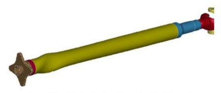
Figure 10 Detailed visualization of the torsional buckling mode
