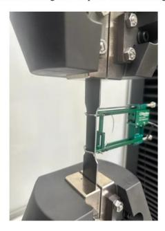
Figure 2 Tensile test machine
