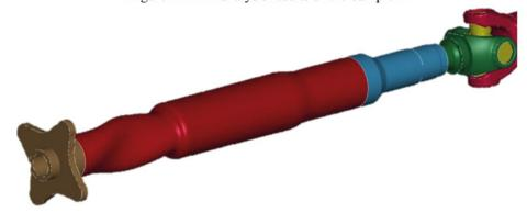
Figure 14 Detailed visualization of the torsional buckling mode
