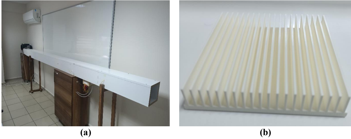
Figure 3. (a) Experimental setup system (b) manufactured plate fin heat sink
