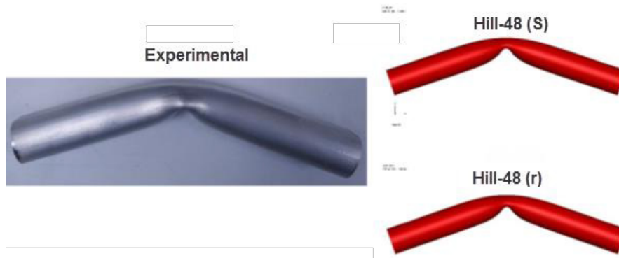
Fig. 10. Comparison of experimental and finite element analyzes of profile with elliptical section geometry with 200 mm span distance and 5 mm punch radius
